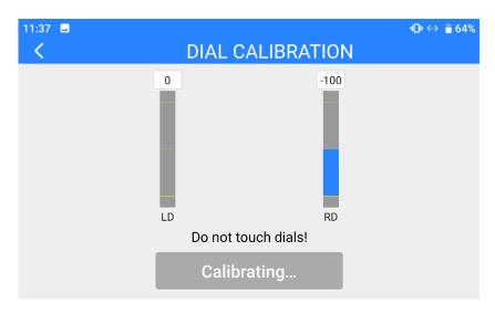
4. Calibration of dial middle points is finished. The next step is to calibrate dial maximum and minimum positions.
