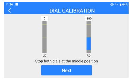
3. According to the tips, if dials' coordinates are not "(0, 0)" when both dials are standstill, it means that dial middle points are displaced. Please touch "next" and do not touch the dials.
