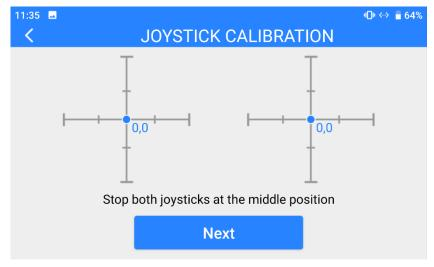
According to the tips, if joystick coordinates are not "(0, 0)" when both joysticks are standstill, it shows that joystick middle points are displaced. Please touch "next" and do not touch joysticks.
