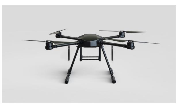
As shown in the figure below, for large multi-rotor drones, the air unit antenna should be placed vertically downwards from the motor base to keep the flat surface of the antenna facing the direction of the remote control. SIVI
